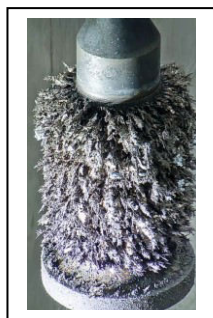
Fig.1: Uranium deposit on solid cathode after Electrorefining operation
